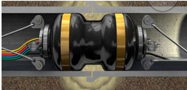
GROUT IS INJECTED AND THE CENTER IS PRESSURIZED
