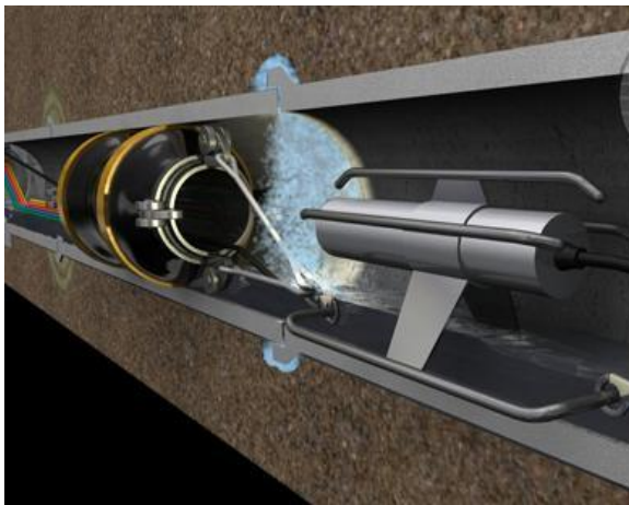
POSITIONING THE PACKER UNIT
