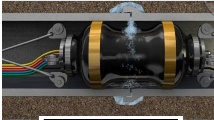
INFLATING THE ENDS OF THE PACKER UNIT
